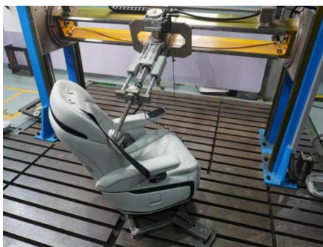
Figure 4. Seat flank stiffness test
