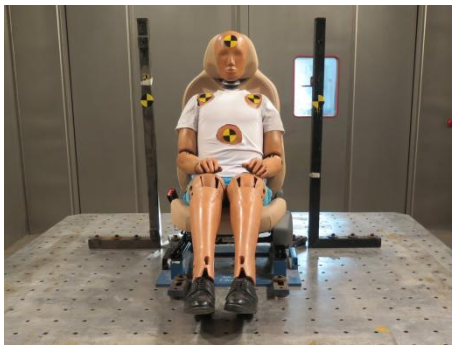
Figure 6. Dynamic body retention test
