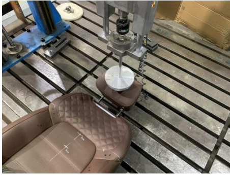
Figure 5. Head restraint retention test
