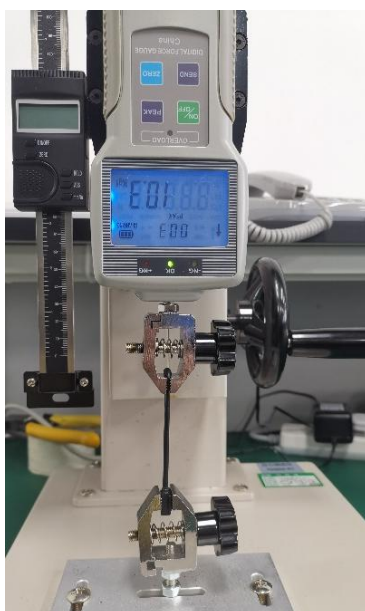
Figure 10. The cable tension value is 126N
