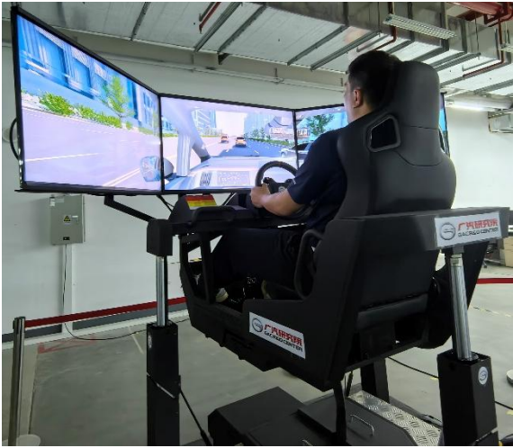
b) Real object of driver-in-the-loop simulator system
