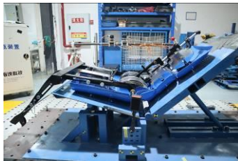
Figure 11 Side view of HPM-II on reclined rigid seat
