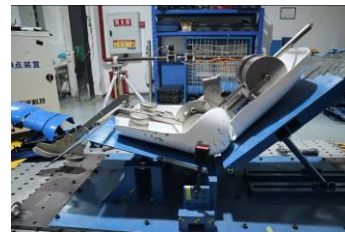
Figure 12 Side view of HPM-I on reclined rigid seat
