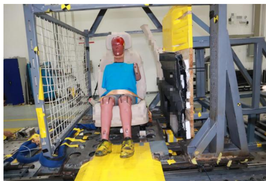
Figure 5. Sled side impact test
