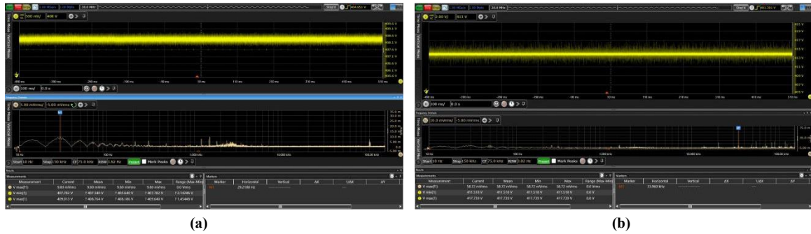
Figure11. Bus voltage of model 3: (a) low temperature DC charging+PTC heating; (b) high temperature DC charging+compressor cooling 图 11.车型三的母线电压: (a)低温直流充电+PTC 制热; (b)高温直流充电+压缩机制冷
