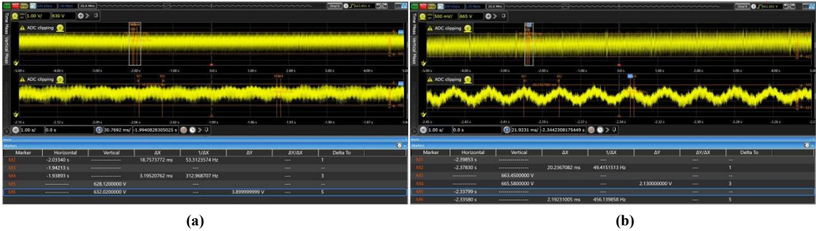
Figure3. Bus voltage of Model 1: (a) under low-temperature DC charging+PTC heating conditions; (b) Under high-temperature DC charging and compressor cooling conditions
