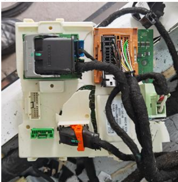
Figure 5. Center electronic module damage after impact test
