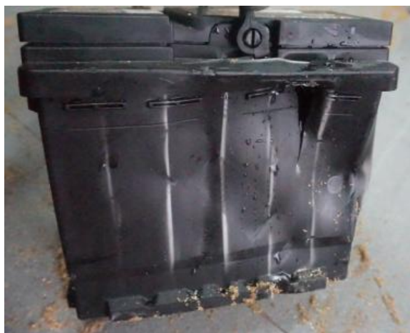
Figure 4. Lower voltage battery damage after impact test
