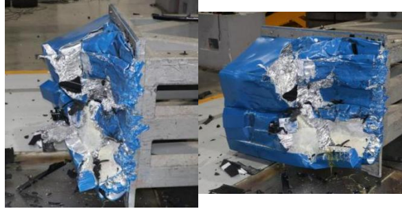
Figure 8. The state of the honeycomb aluminum after the ODB test (No. 4)
