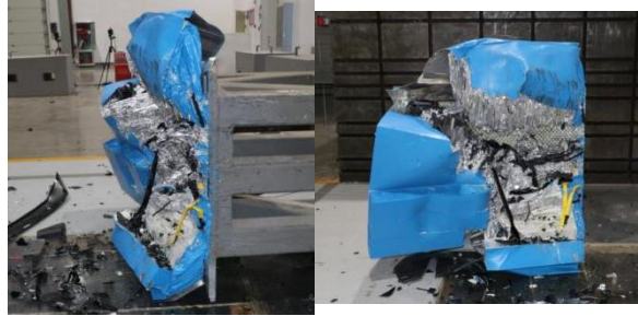
Figure 7. The state of the honeycomb aluminum after the ODB test (No. 3)
