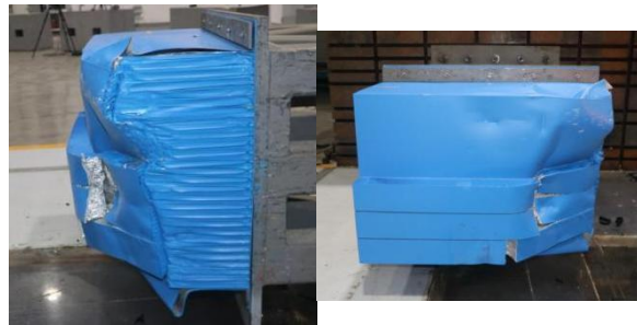
Figure 5. The state of the honeycomb aluminum after the ODB test (No. 1)
