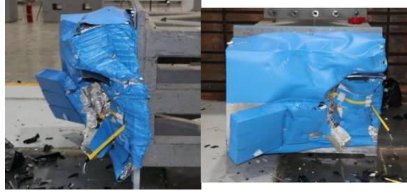
Figure 6. The state of the honeycomb aluminum after the ODB test (No. 2)
