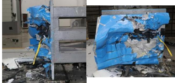
Figure 9. The state of the honeycomb aluminum after the ODB test (No. 5)
