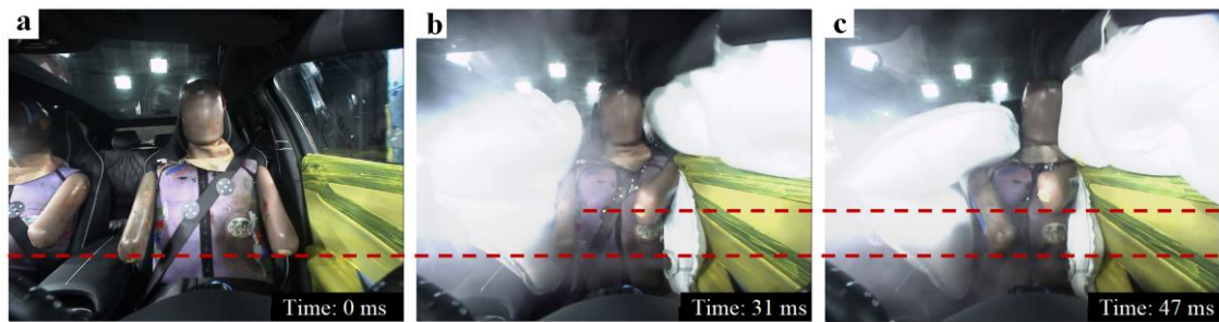
Figure 2. Dummy response in side pole impact for a specific vehicle. (a) Dummy state of pre-crash, (b) Dummy state at 31 ms, (c) Dummy state at 47 ms.
