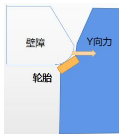
Figure 6. Schematic diagram of small offset slip
