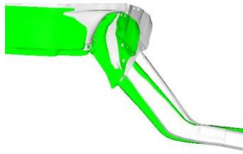
**Figure 9. Transform of engine room side rail(Gray-base, Green-case)**
