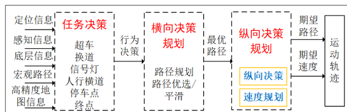
Figure 1. Smart car motion planning diagram
