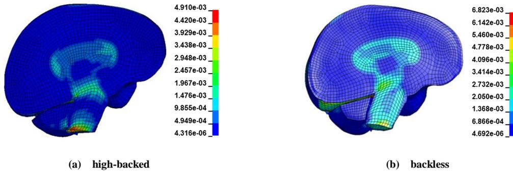
Figure12 Brain Shear Stress Clouds
