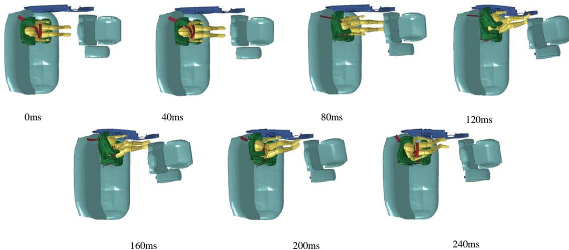
Figure 6 Occupant Kinematic Response (high-backed)
