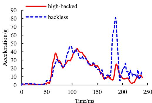
**Figure8 Head Resultant Acceleration**
