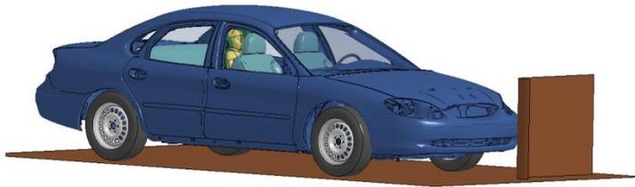
Figure 4 Small Overlap Frontal Impact FE Model
