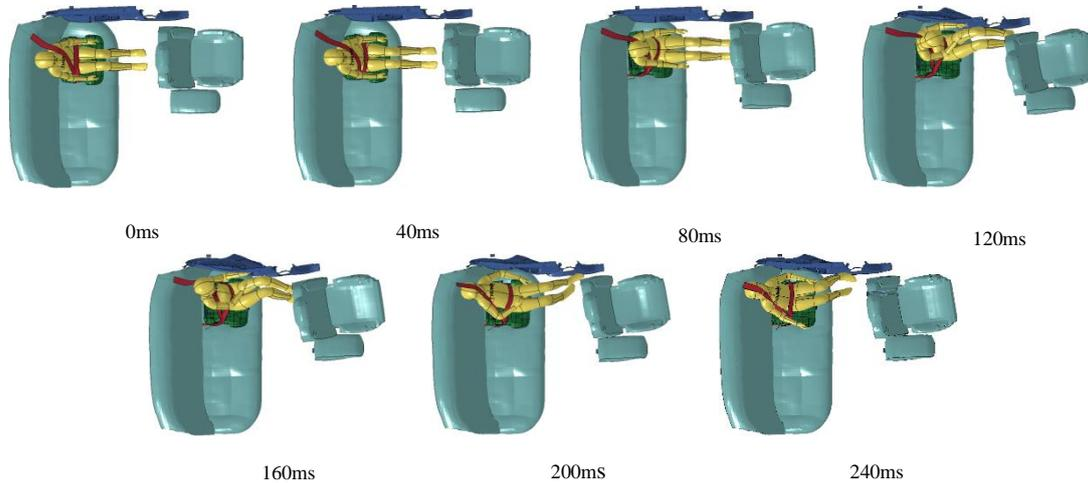
**Figure7 Occupant Kinematic Response (backless)**
