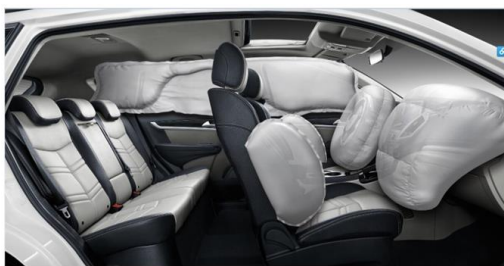
Figure 1. Side air curtain expansion system
