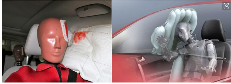
Figure 5. The occupant makes contact with the side air curtain
