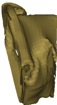
Figure 6 .The distortion of crash-box is deficient
