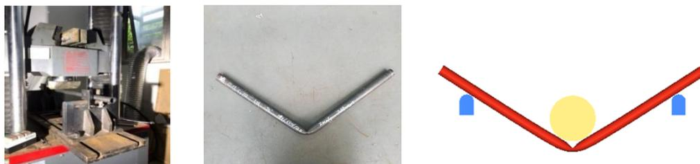
Figure 6. Curve: Static test and simulation of door beam deformation
