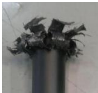
Figure 5. Pipe collision results
