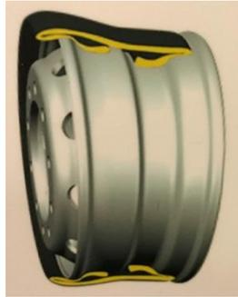
Figure 2.1 The damaged tires were torn and detached from the rim
