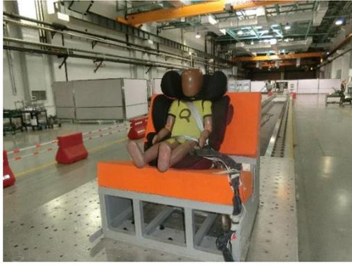
Figure 8. three-point seat belt fixed in frontal collision
