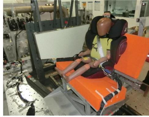
Figure 9. three-point seat belt fixed in side collision
