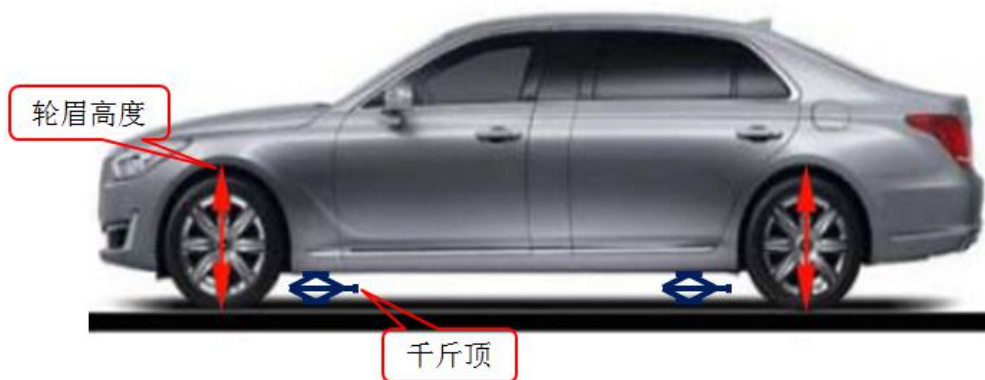
Figure 4. The vehicle being uplift by jack
