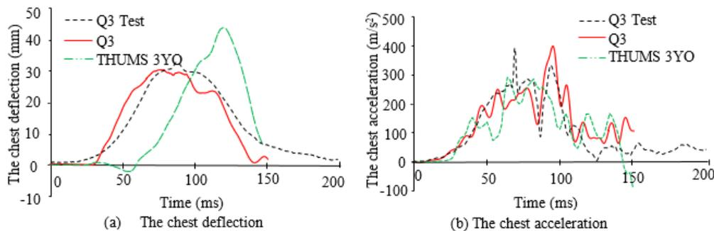
Fig. 7 the chest deflection and chest acceleration of the Q3 and THUMS 3YO in the impact shield CRS A
