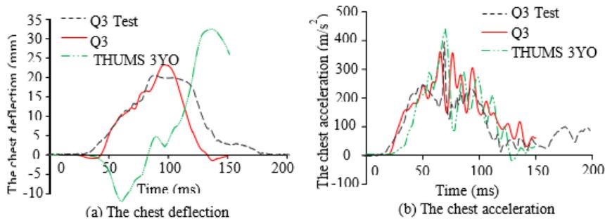
Fig. 8 the chest deflection and chest acceleration of the Q3 and THUMS 3YO in the impact shield CRS B
