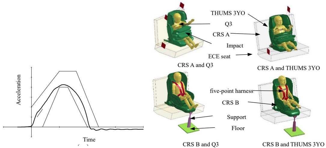
Fig. 3. Acceleration of the sled with UN R129 corridor. Fig.4. Impact shield and five-point harness CRS simulations set-up
