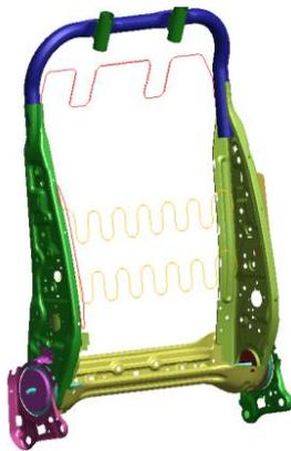
Figure 2. The backrest insert frame structure seat①、②
