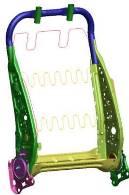
Figure 3. The backrest insert frame structure of seat③
