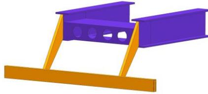
Figure9. Diagram: the vehicle rear underride protection device ( II )
