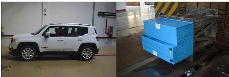
Figure 6. SUV and barrier before crash test
