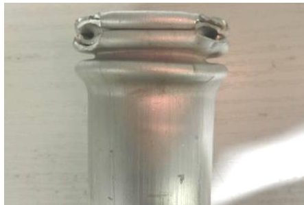
a) Crushing form (4 induced holes)
