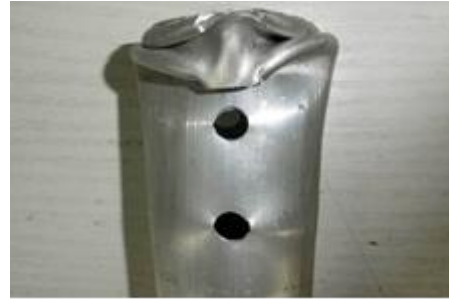
b) Crushing form (2 induced holes)
