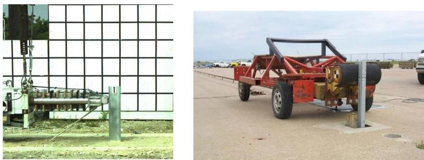
Figure 1. pendulum test and bogie test
