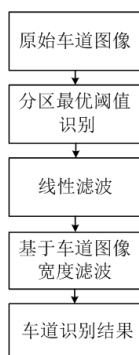
Fig. 1 Lane recognition process within each image section
