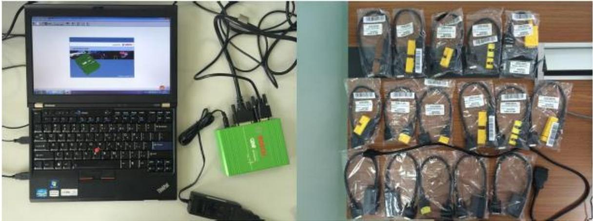
Figure 5. CDR devices and connecting cables
