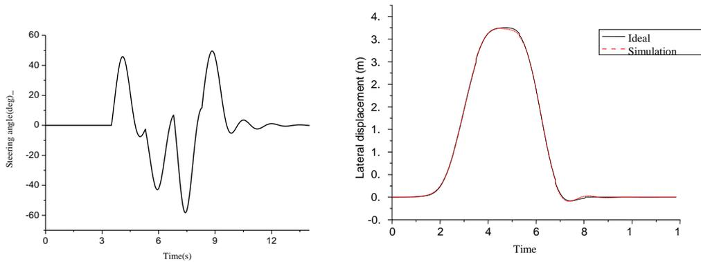
**Figure 15.**The steering angle and the lateral displacement of double lane change test
