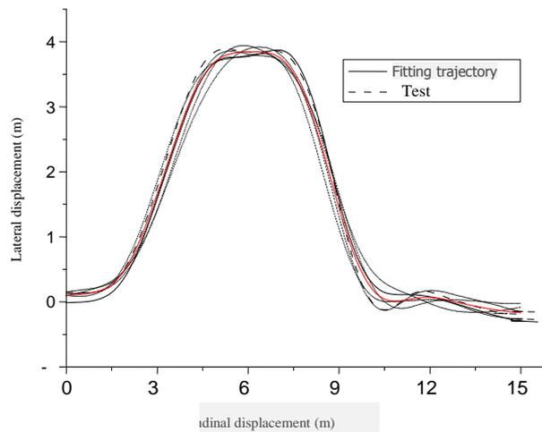
Figure 13. The fit trajectory and the measured trajectory of double lane change test
