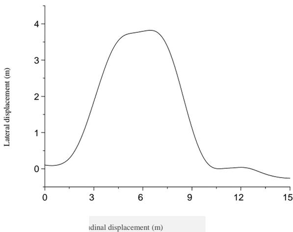
**Figure 17.The trajectory of double lane change test**
