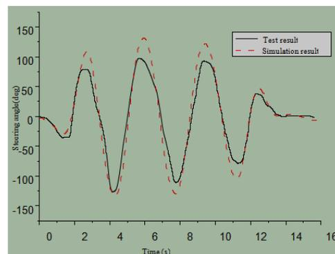
**Figure 20.The steering angle comparison of test result and simulation result**
