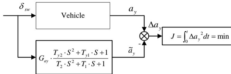
Figure 3. The identification process of vehicle parameters
