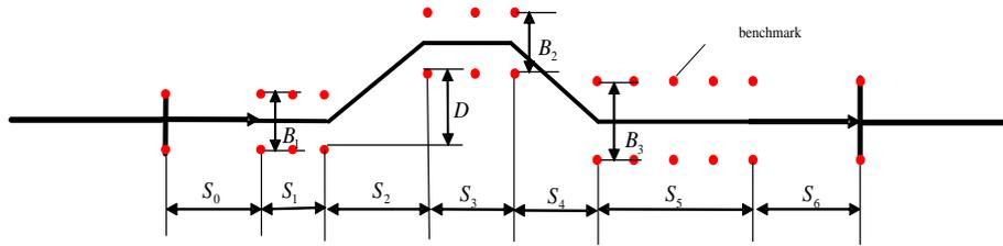
Figure 11. The site layout of double-lane change test
