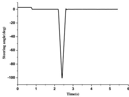
Figure 4. Pulse signal of steering angle
