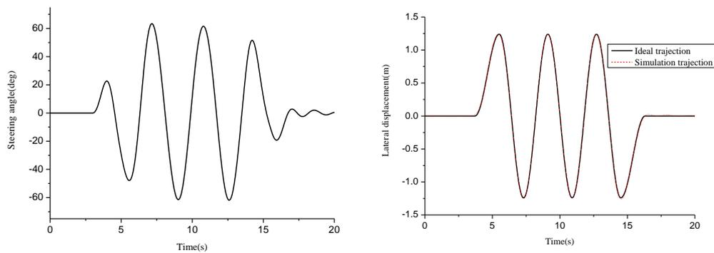
**Figure 16.**The steering angle and the lateral displacement of slalom test
