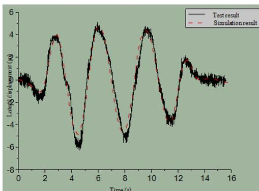
**Figure 19.The lateral displacement comparison of test result and simulation result**
