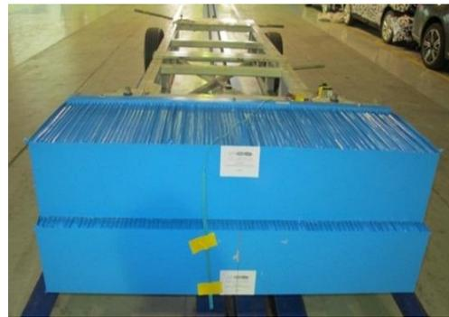
Figure 12. Deformable barrier
