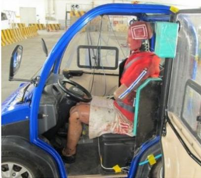
Figure 11. Dummy position adjusting
