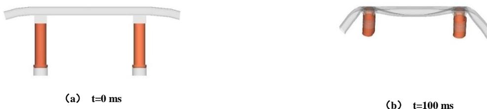
Figure 13. Turnup pipe deformation contrast figure
