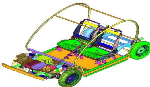
Figure 23. The electric car vehicle finite element model
