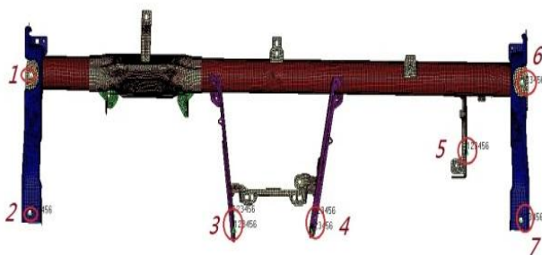
Figure 4. Meter version beam assembly constraints 图 4.仪表板横梁总成约束位置
