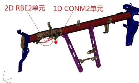
Figure 3. Version of the finite element model of beam assembly 图 3.仪表板横梁总成有限元模型
