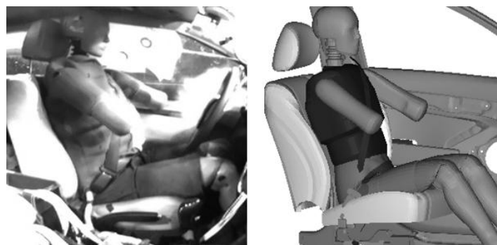
Figure 5. Occupant kinematics and airbag deployment in both test (left) and simulation (right) at 30ms
