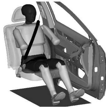
Figure 2. The occupant simulation model
