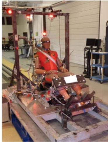
**Fig 1. THOR dummy sled test**
