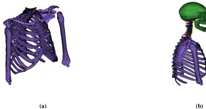
Figure 2. thorax model (a) and HBM-Head-Neck FE model (b)
