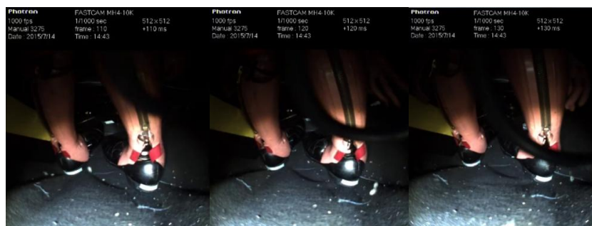
(g) 110ms (h) 120ms (i) 130ms Figure 4. The passenger foot and leg movement in the process of collision process
