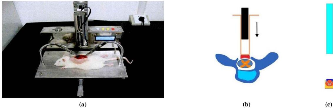
Figure 5. (a) Hammer impact experiment of rat's spinal cord; (b) Schematic diagram of hammer impact experiment of rat's spinal cord; (c)The simulation of hammer impact model
