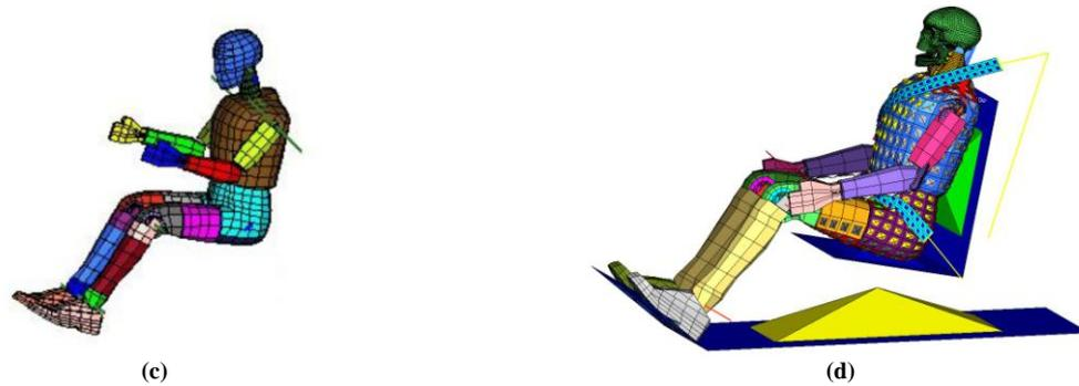
Figure 7. (a)Sipne cord assembled with the cervical vertebra; (b) Fundamental FEM of head-neck complex that contains muscle geometry feature and active response of muscle; (c) Hybrid III dummy model; (d) Hybrid FEA model
