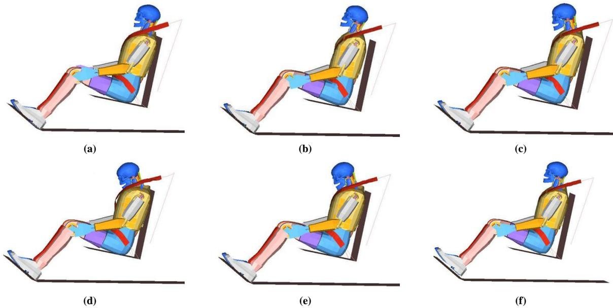
Figure 13. Hybrid dummy model's movement process during frontal crash. (a) Initial state; (b) Leaning state of body; (c) Forward flexion of the neck; (d) Excessive flexion of neck; (e) Body resilience status; (f) Final state.
