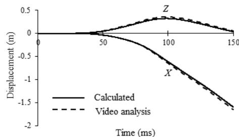
Figure 12. Comparison of the calculated result and the result from video analysis of sled test
