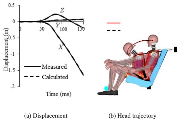
Figure 6. Comparison of actual head trajectory and head trajectory calculated from data from the accelerometer in the rear seat passenger's head
