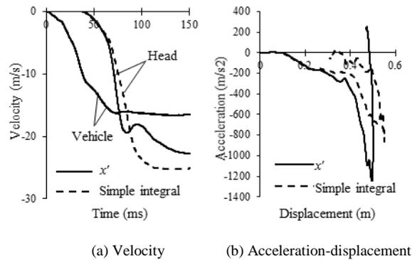
**Figure 7. Velocity-time and acceleration-displacement history of the dummy's head from calculation (including dummy rotation) compared to these from simple linear acceleration integral (rear seat)**
