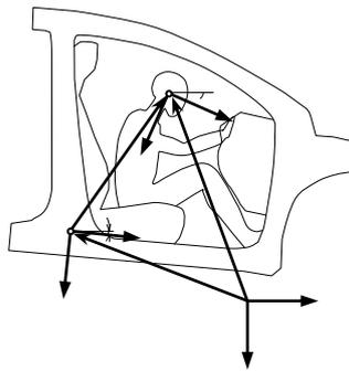
Figure 1. Global coordinate system, and the local coordinate system of the passenger compartment and dummy's head
