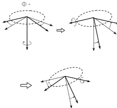
Figure 4. Transformation from the global coordinate system to the local coordinate system using Euler angles
