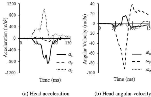
Figure 5. Data obtained from the accelerometer located in the CG of the rear seat passenger's head
