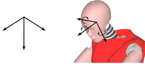
Figure 2. Detailed view of the global coordinate system and the dummy's head local coordinate system
