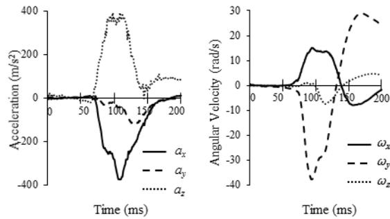
(a) Head acceleration (b) Head angular velocity
