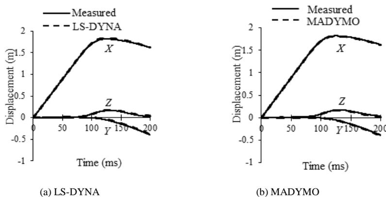
Figure 13. Head displacement in original crash simulation compared to LS-DYNA and MADYMO simulations using the head's acceleration and angular velocity
