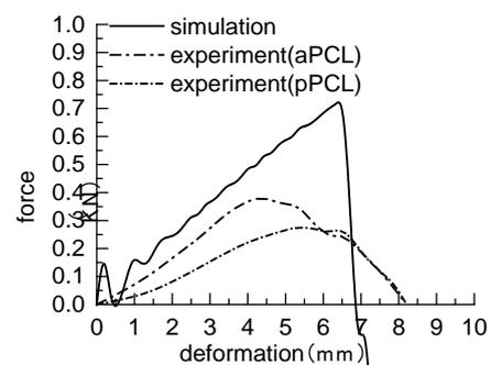
Figure 13: verification of PCL at high strain rate loading
