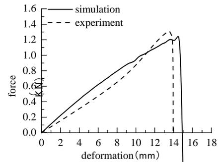
Figure 8: verification of MCL at low strain rate loading
