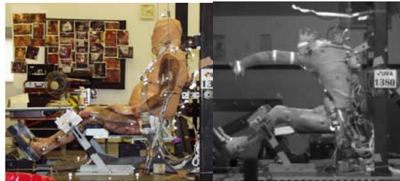
Figure 1:Initial position (left), and video capture at the time of maximum forward head excursion (right) from one of the tests that formed the basis for these simulations.
