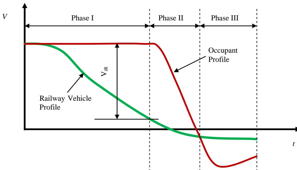
Figure 6: Railway vehicle and occupant velocity history
