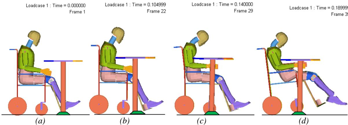
**Figure 10: Wheelchair and occupant kinematics for fixed bay table. (a) start of primary collision; (b) chest contacts table edge first; (c) maximum chest deflection; (d) lower body submarines.**
