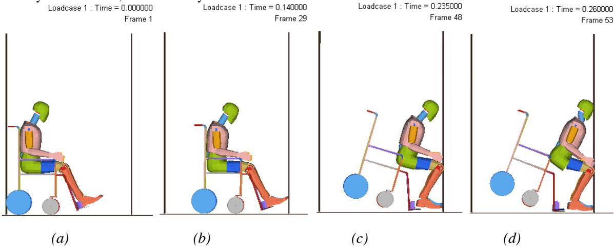
**Figure 9: Wheelchair and occupant kinematics for partition. (a) start of primary collision; (b) feet contact the partition first; (c) knee contact with partition; (d) head contact with partition loads the neck**
