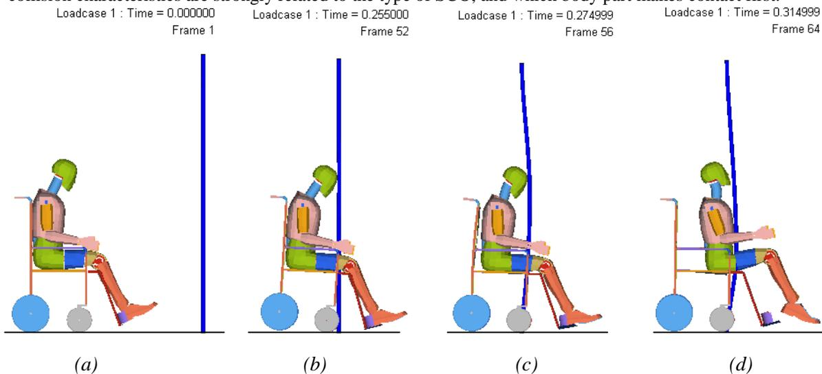
**Figure 8: Wheelchair and occupant kinematics for grab pole. (a) start of primary collision; (b) head contacts the grab pole first; (c) head contact loading deforms grab pole; (d) pelvis contacts the grab pole.**
