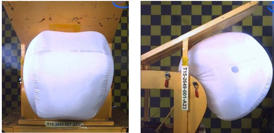
Figure 3. Front view (left) and side view (right) of PAB static deployment in vehicle environment 图 3. 乘员气囊的工装环境下静态点爆试验正面图（左）和侧面图（右）
