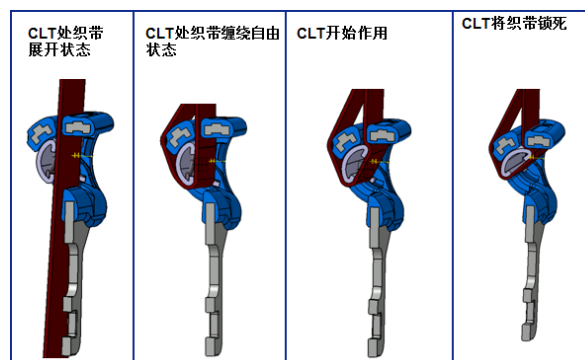
Figure 6. a CLT working principle illustration
