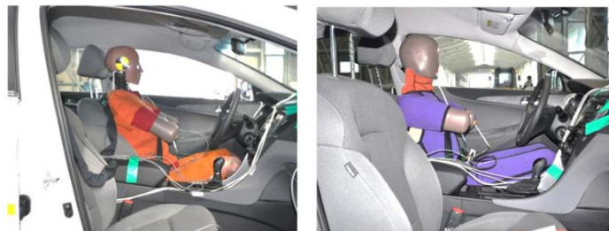
Figure 9. Dummy seated in the mid-size car
