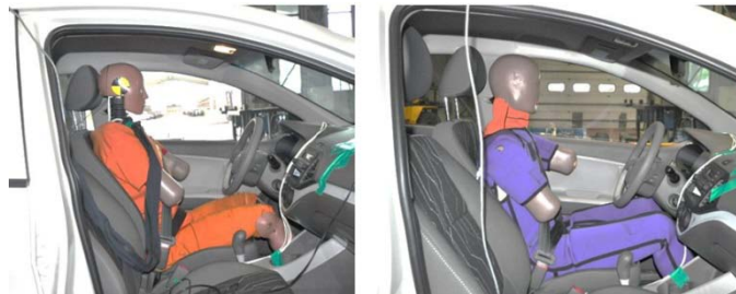
Figure 8. Dummy seated in the compact size car
