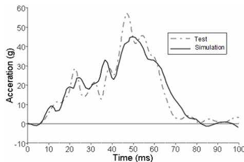
Fig. 2 Comparison of the vehicle acceleration curve (at B pillar) in experiment and Simulation
