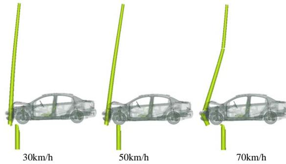
Fig. 6 The dynamic response of collision at different speeds
