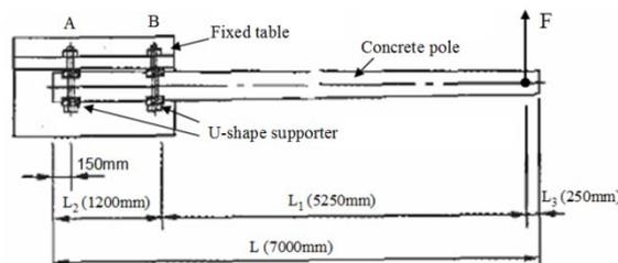
Fig. 3 The cantilever deflection diagram of experimental setup (unit: mm)
