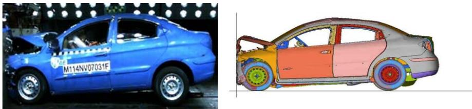
Fig. 1 Comparison of deformation between crash test and simulation
