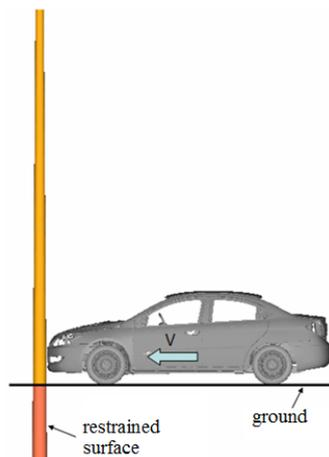
Fig. 5 the simulation setup of car-pole collision
