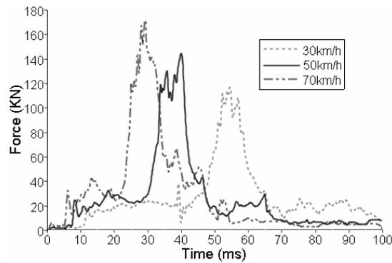
Fig. 7 Pole fractures at different speeds
