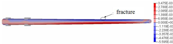
Fig. 4 The stress contour of cantilever deflection test at failure time (unit: GPa)
