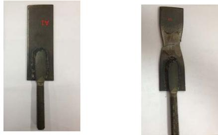
Figure 3 Tensile test of the conjunction
