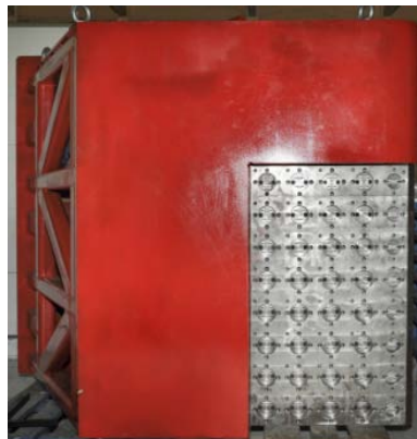
Figure 5. Small overlap barrier acquisition system
