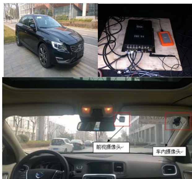
Figure 1. Experiment vehicle Volvo S60L and data collection equipment
