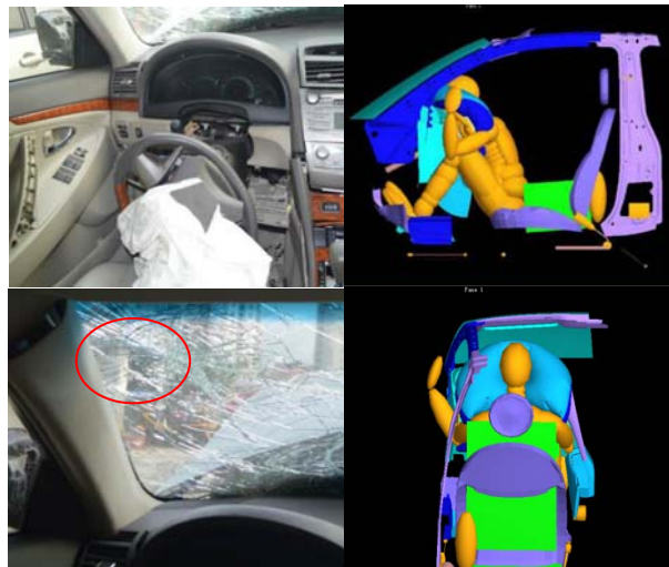
Figure 6 Comparison between Reconstruction Results and Real Situation inside Vehicle of Case 6
