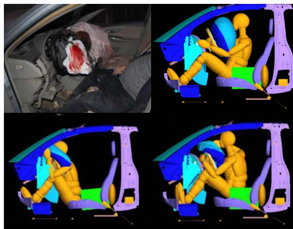
Figure 5 Comparison between Reconstruction Results and Real Situation inside Vehicle of Case 2
