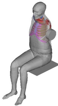
Figure 1. ISO view of current thorax FE model in impactor loading conditions
