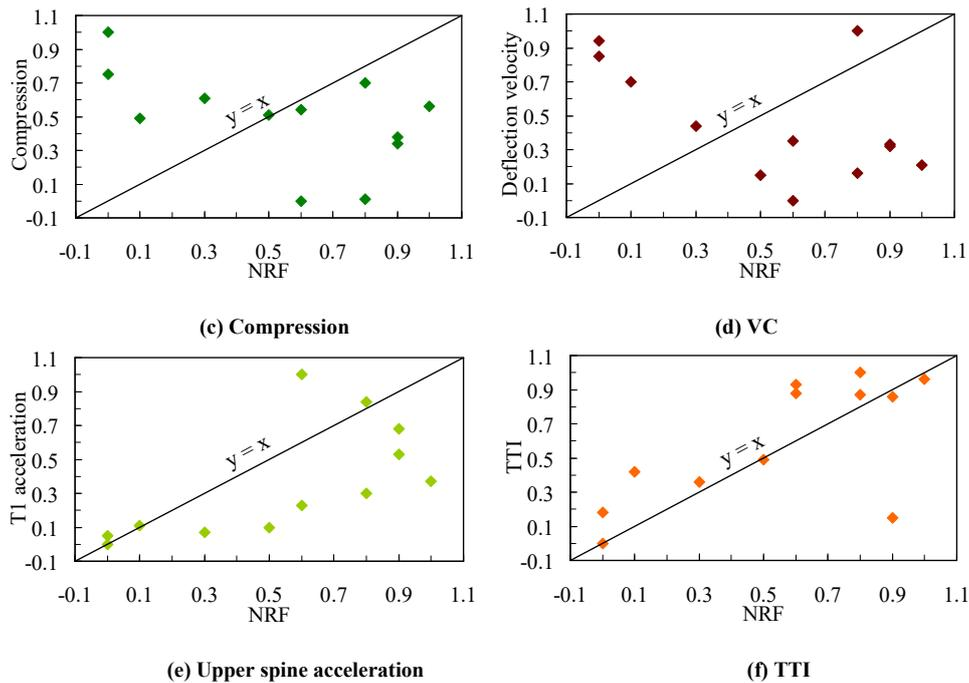
Figure 6. Normalized NRF as functions of the various injury criteria
